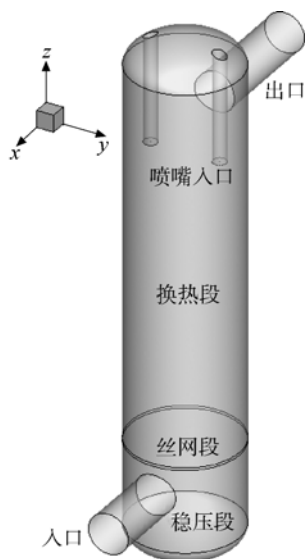
图 16 气氮调温器结构 Fig. 16 Structure of the \text{LN}_2 -spray temperature-adjusting system
